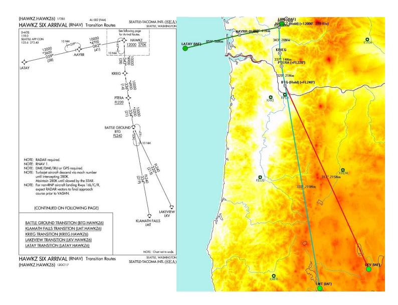
The values are OK (except the magnetic heading, it's always the same, the magvar for the map is the local one, but the FMS of the aircraft keep the value of the airport of the procedure...) here you will understand and categorize the error.
